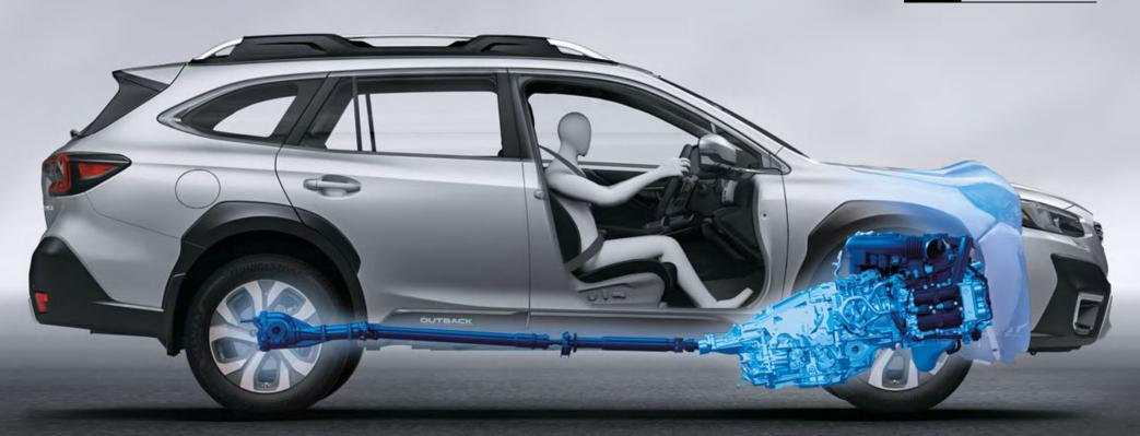
Designated crumple zones direct impact energy away from the ring-shaped passenger safety cell, while the Boxer engine is designed to slide below the cabin in a severe frontal collision.
