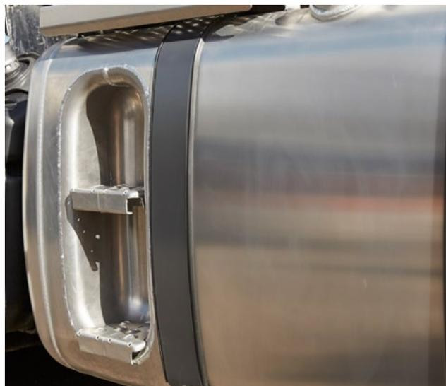
**Flexible tank variants.** Within the same tank cross-section different tank capacities can be combined on the left and right-hand side. This applies to diesel and AdBlue<sup>®</sup> tanks as well as to combination tanks.
