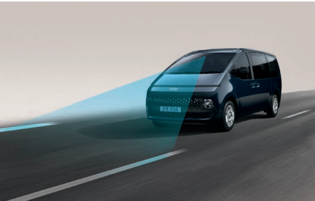
Lane Keeping Assist (LKA) A front view camera detects lane markers and road edges helping prevent unintentional lane departures. When the vehicle strays from its lane (or road), the system sets off a visual and sound alarm and automatically steer the vehicle to prevent it from moving out of its lane (or road).
