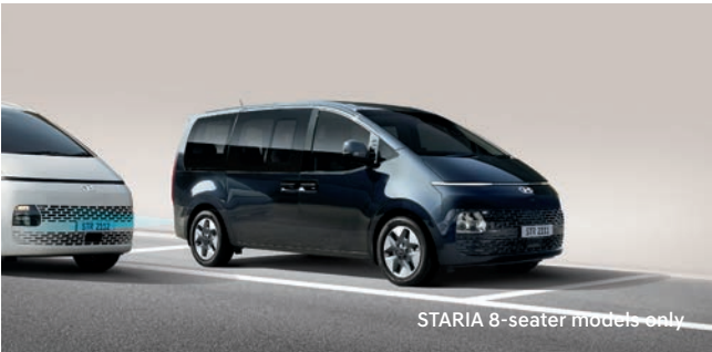
Safe Exit Assist (SEA) When the occupant opens the door to exit the vehicle after a stop, if an approaching vehicle from the rear side is detected, the function provides a warning. The function also helps keep the rear door closed through operation of the power sliding door on STARIA Limited models.
