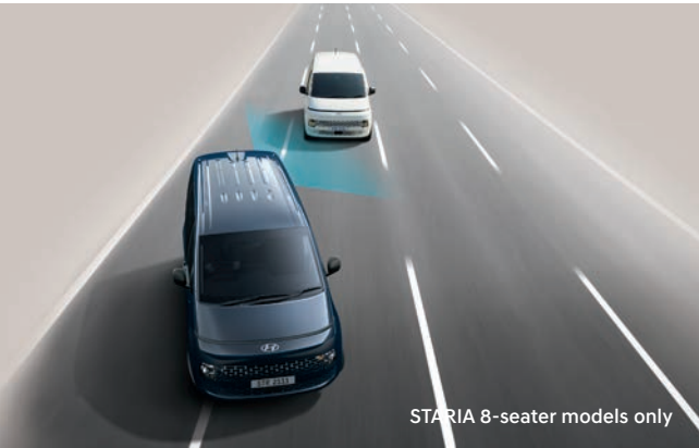
Blind-spot Collision Warning (BCW) When operating the turn signal switch to change lanes, if there is a risk of collision with a rear side vehicle, the system provides a warning.
