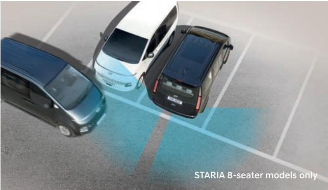
Rear Cross-traffic Collision Warning (RCCW) RCCW warns of the approach of a vehicle across the rearward path when reversing.
